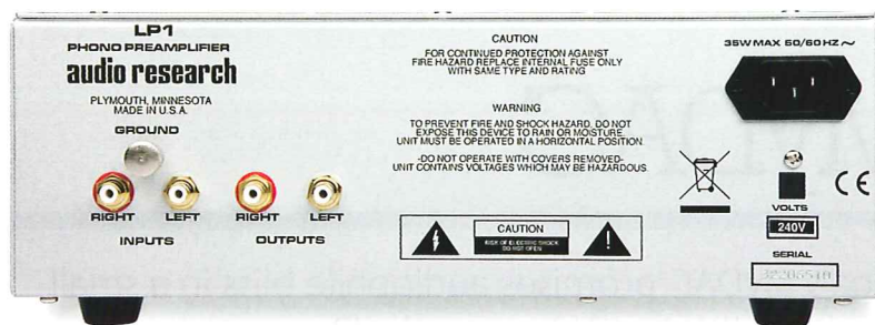
ABOVE: Rear panels do not come much simpler – just one pair of RCA phonos for input and another for line-level connection to a separate amp/preamp. There are no user-adjustable gain or loading options available here
